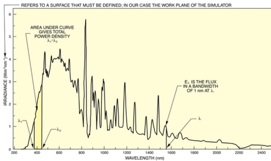
Fig. 1 Example of Oriol Solar Simulator spectral output curves .
